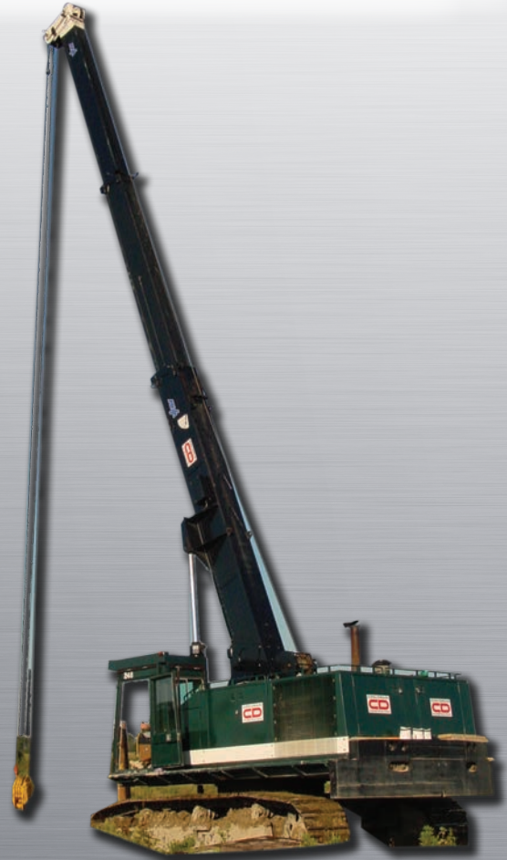
CRANE FOR CAT 245 - CAPACITY OF 5 TONS @ 60' BOOM
