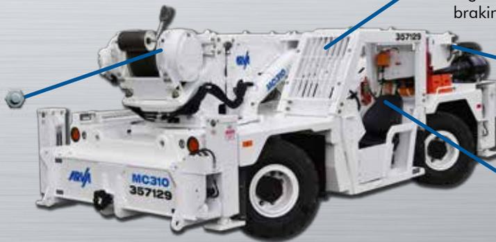
Designed for mining conditions and regulations, including ROPS/FOPS, dual braking and approved fire suppression system.
