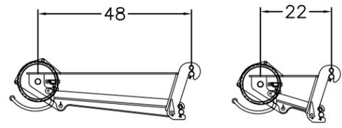
SHEAVE ATTACHMENT CAN BE DESIGNED IN ALMOST ANY SHAPE OR SIZE, TWO EXAMPLES ARE SHOWN CUSTOMER TO SPECIFY WINCH HOOK CONNECTION; BECKETT AND HEADACHE BALL VERSUS SWAGED END, AS SHOWN
