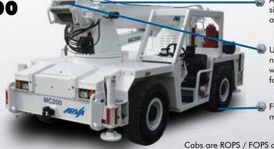
ARVA cranes have more than twice the boom side loading capability than the competition to assist with swinging heavy loads in rough terrain.
