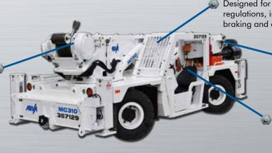
Designed for mining conditions and regulations, including ROPS/FOPS, dual braking and approved fire suppression system.
