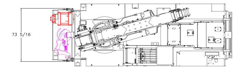
SECONDARY WINCH AND SHEAVE ATTACHMENT TRAVEL/STORAGE\_ LOCATION ON 6600 LB CAPACITY CARRY DECK
