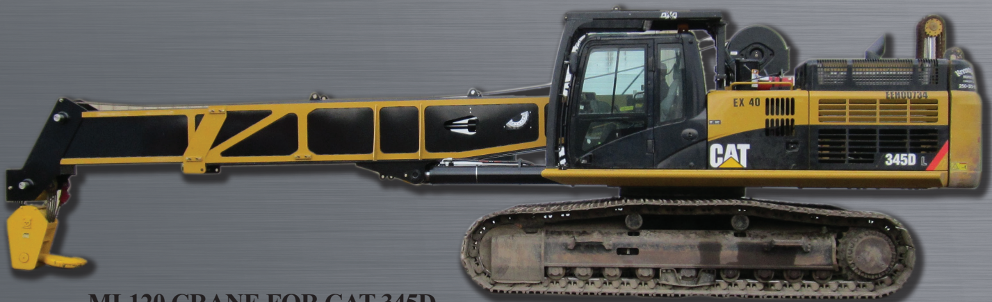
ML120 CRANE FOR CAT 345D - CAPACITY OF 83 TONS @ 7' BOOM
